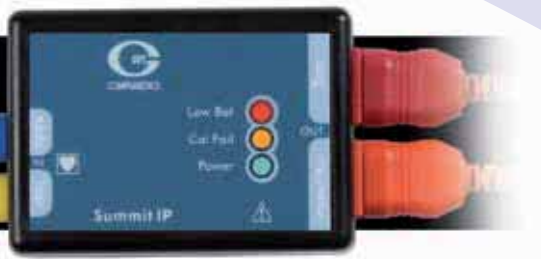
Summit IP™ – Respiratory effort sensor system using true inductive plethysmography
